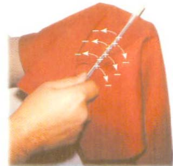
FIGURE 15.2 When a glass rod is rubbed with silk, electrons are transferred from the glass to the silk. Because of conservation of charge, each electron adds negative charge to the silk, and an equal positive charge is left behind on the rod. Also, because the charges are transferred in discrete bundles, the charges on the two objects are \pm e , \pm 2e , \pm 3e , and so on.
